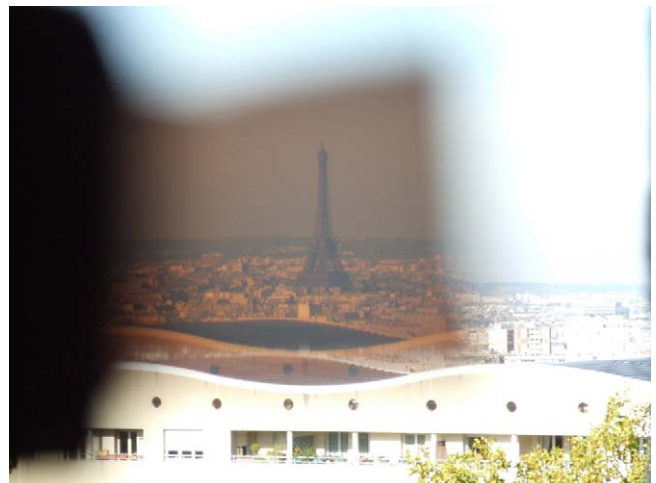
Fig. 9. The Eiffel Tower observed through one of our best polycrystalline alumina sample (thickness = 2.8 mm).
